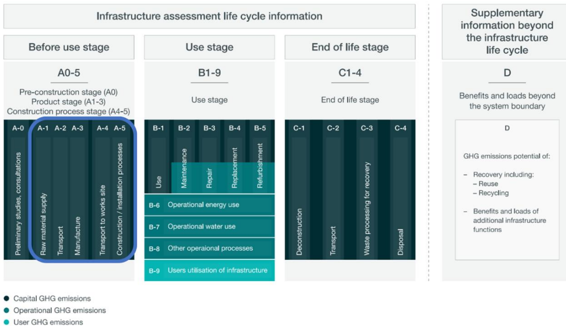
Figure 8.1: PAS 2080: 2016 Lifecycle stages for infrastructure 60
